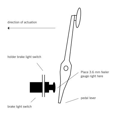
Brake lights must flash up at latest after 12 mm.
